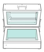
Insert your mask(s) inside the ECD. If your mask has overlapping materials, fold it open so the ECD light can reach all its surfaces.
